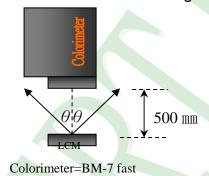
To be measured at the center area of panel with a viewing cone of 1° by Topcon luminance meter BM-7, after 10 minutes operation (module)
