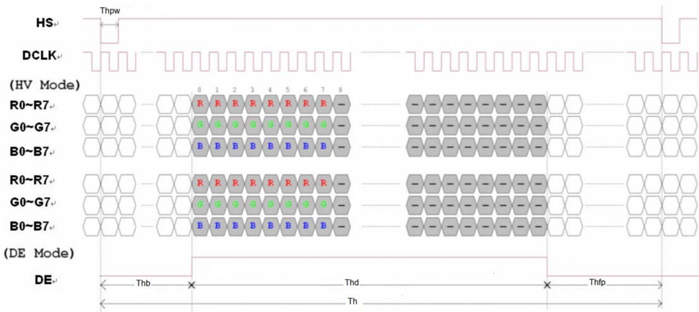
Horizontal input timing diagram
