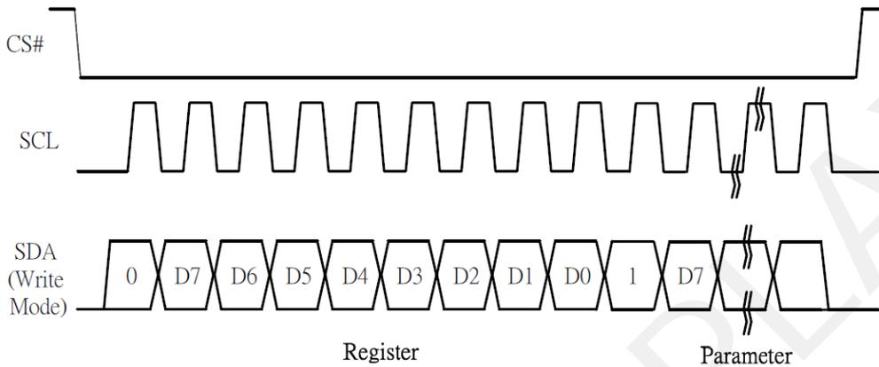
Figure 3.5-3: Write procedure in 3-wire SPI mode
