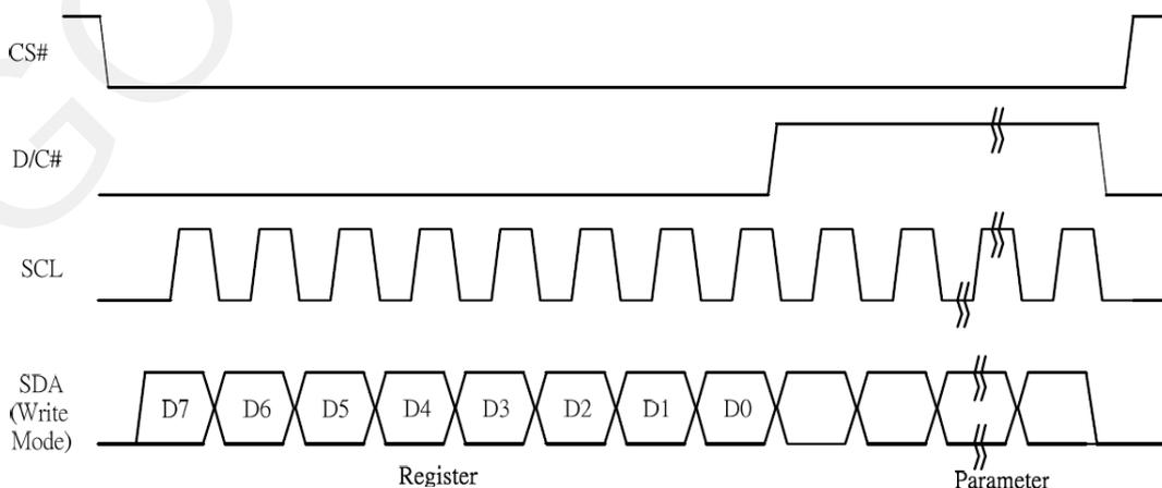
**Figure 3.5-1: Write procedure in 4-wire SPI mode**
