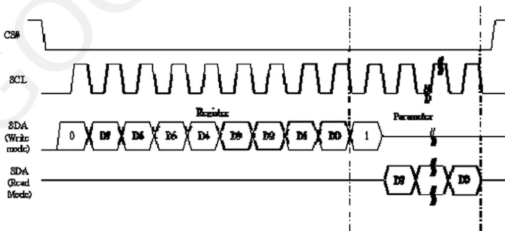
Figure 3.5-4 Read procedure in 3-wire SPI mode
