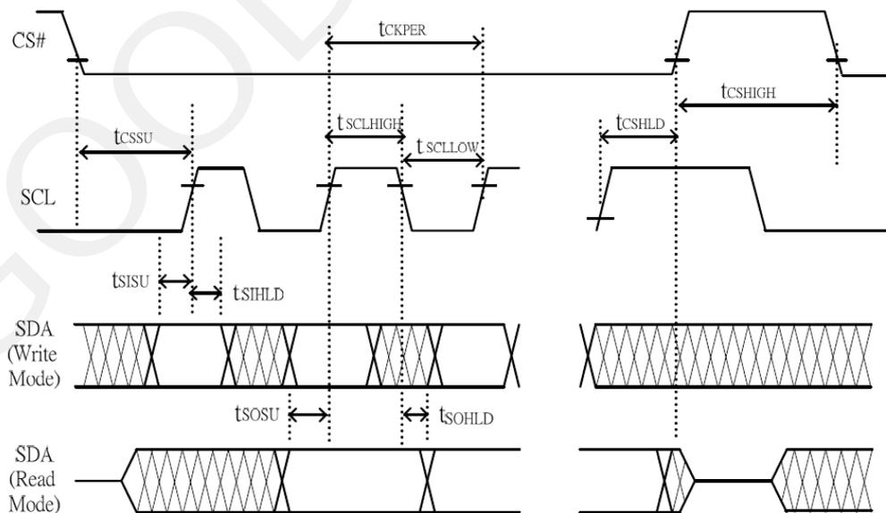
Figure 3.3-1: SPI timing diagram
